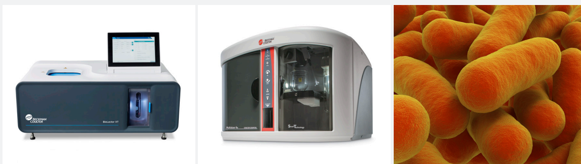
FIGURE 1: The BioLector microbioreactor and the Multisizer 4e Coulter Counter can be used to monitor E. coli cultures.
